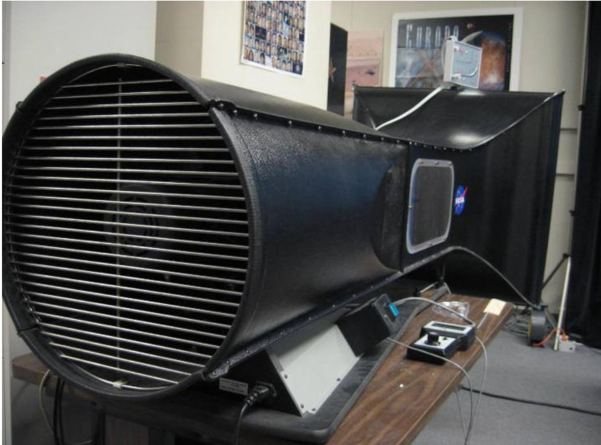
Airflow through this tunnel is from right to left. The largest part, at the right of the tunnel, is called the **bellmouth**. For this tunnel, the flow straighteners are placed at the entrance to the bell mouth as shown here.
